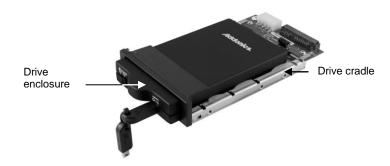
**Step 1:** Connect a SATA cable to the 7-pin SATA data connector to the SATA interface of the cradle.
